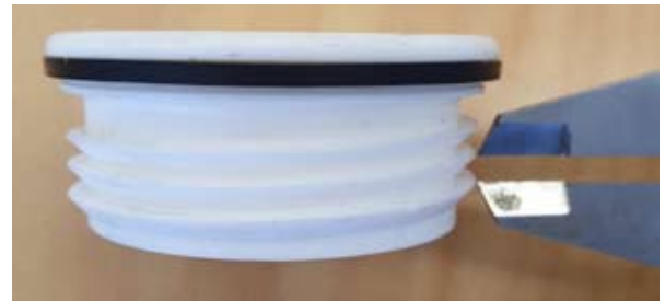
Pitch of the thread (distance between threads)
