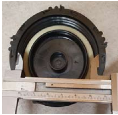
Inner diameter of cap or other female thread (e.g. drum)
